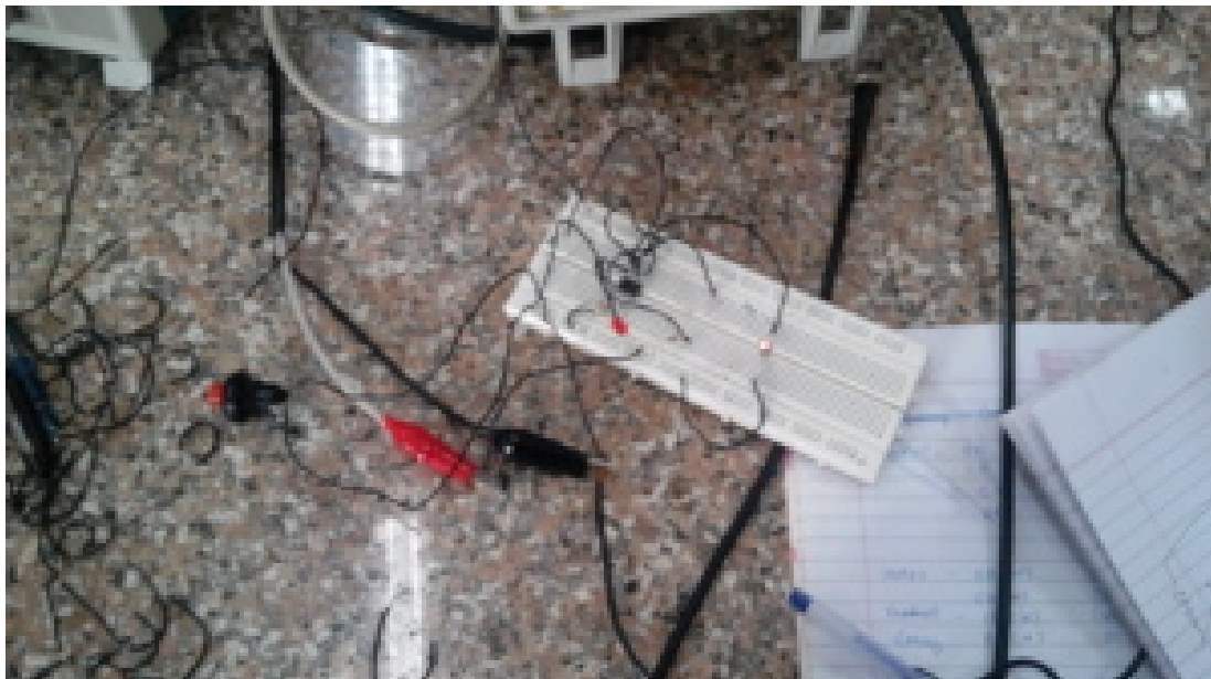
The Circuit for Monostable Multivibrator
